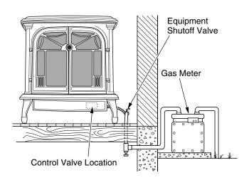
Figure 11 - Checking Gas Joints on Natural Gas Unit
